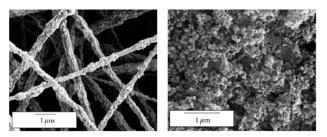
Fig. 5 – SEM micrographs showing the morphological features of electrospun fibers (left) and spincast films (right) of PHB blended with TiO<sub>2</sub>. Reprinted from reference<sup>75</sup> with permission from Hindawi Publishing Corporation.
