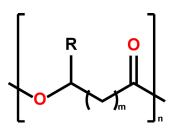
Fig. 1 – Generic structural formula of PHAs. The integer m typically has the value of 1 (with the exception of 4-hydroxy-alkanoates such as 4-hydroxybutyrate), the integer n quantifies the degree of polymerization.
