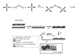
Fig. 3 – Top: Crosslinking of polymer chains with a bisazide (BA) under UV irradiation. Bottom: Multi-step photolithographic processes based on P(HB-HV). Reproduced in part from reference<sup>14</sup> with permission of The Royal Society of Chemistry.
