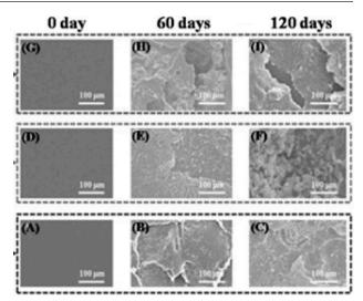
Fig. 4 – SEM images of the morphology of PHA composites after 0, 60, and 120 days of degradation. A-C: pristine PHA, D-F: PHA crosslinked with cellulose actetate, G-I: PHA grafted on acrylic acid/cellulose acetate. Biodegradation by Acetobacter pasteurianus can be monitored by the erosion in the films. Reprinted from reference<sup>66</sup> with permission from Elsevier.
